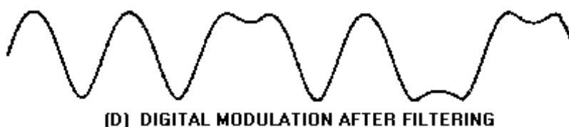
Figure 2-26D.—Simulated phase-shift keying. DIGITAL MODULATION AFTER FILTERING.
