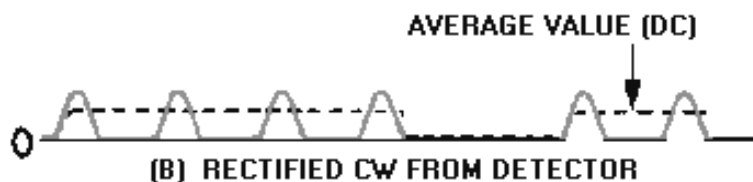
Figure 3-1B.—Cw demodulation. RECTIFIED CW FROM DETECTOR.
