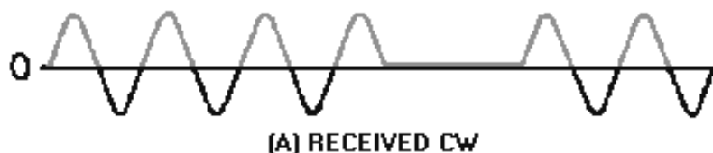
Figure 3-1A.—Cw demodulation. RECEIVED CW.
