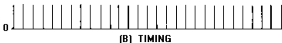
Figure 2-47B.—Pulse-frequency modulation (pfm). TIMING.
