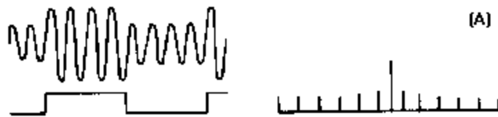
Figure 2-29A.—Various square-wave modulation levels with frequency-spectrum carrier and sidebands.
