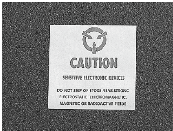
Figure 3-31.—Warning symbols for ESDS devices.
