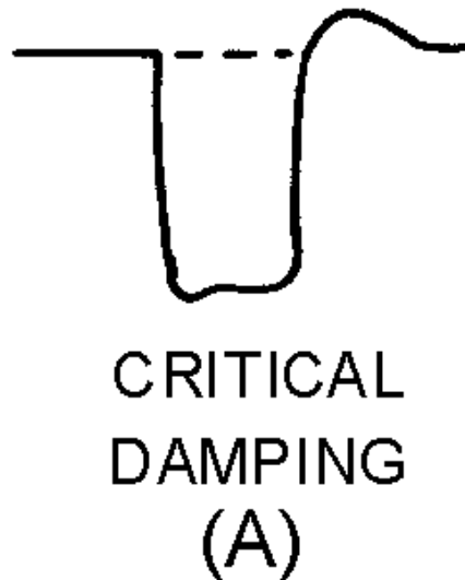
Figure 3-36A.—Waveform damping. CRITICAL DAMPING.
